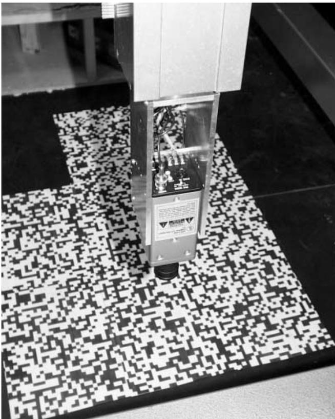
Fig. 10. View of robotic gantry, showing camera head and visual texture on the floor
