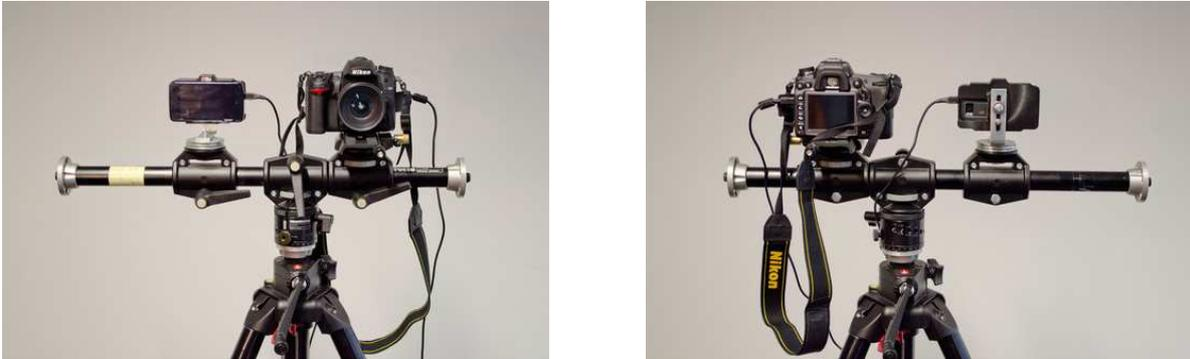
The no parallax requirement implies that the second camera must take the position of the first when shooting. A practical solution offering high precision is shown in Figure 3. By rotating the accessory arm by 180 degrees one camera can take the position of the other. In the case of ideal camera adjustment the entry pupils of both cameras are matched by the rotation.
