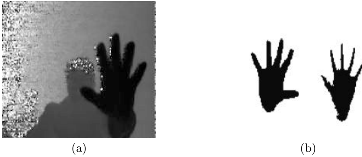
Fig. 3. (a) Frame from a near-range ToF camera (PMD CamBoard Micro): note the large amount of noise in the background and near the edges of objects. (b) Motion artifacts: the moving hand (right) has thinner fingers than the static hand (left).
