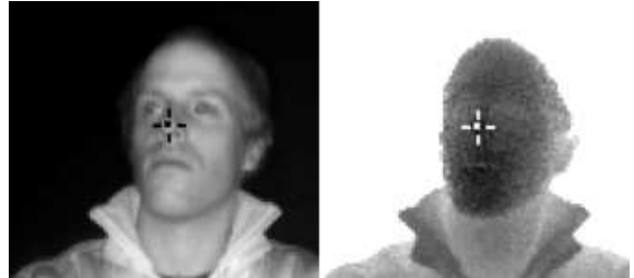
Figure 5. Example nose-detection results shown on ToF-intensity (left) and ToF-range image (right); detection error rate is 0,03 [4]. A MESA SR3000 cameras has been used.
