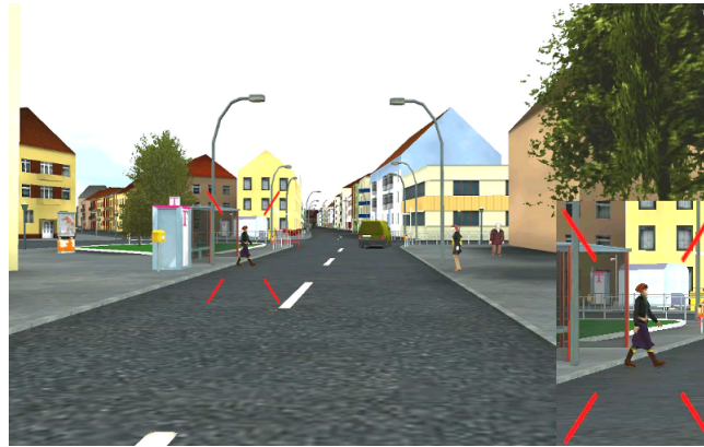
Fig. 1: Simulator scene. Because the driver is looking away (red 3D marker), the pedestrian beginning to cross the street is highlighted with a gaze-contingent cue. Bottom right: gaze-contingent cue enlarged for better visibility (not shown during the experiment.)
